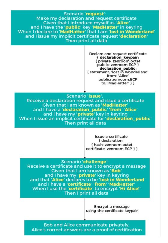
At last, below is a diagram showing again the code and the data-structures of the credential authentication mechanism implemented following the Coconut paper (Sonnino et al., 2018) and illustrating the flow of request, issue and publication of credentials outlined in this graph:
