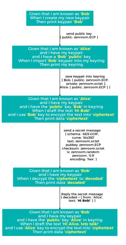
This simplified flow diagram shows **actual Zencode** that can be executed, higlighting variables that are normally just surrounded by single quotes. Between each code block, which is executed asynchronously as required and at different times, there is a schema which indicates the shape of data in output.
